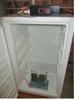
The Inveterate Inventor had an earlier fridge that had been used for many years as a warming cabinet. The fridge had the thermostat sensor loose in the cabinet with their lead running to the control unit via the fridge door.
